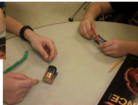
Building electromagnetics using wire, nails and batteries. Watch the wire it can get hot.
