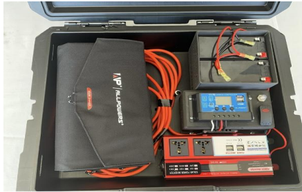
1st Prototype: Solar Suitcase Suitcase lacked durability. Dual lead-acid batteries were heavy with low capacity. PWM charge controller proved inefficient. Inverter underperformed and overheated.
